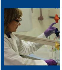
The fume hood is often the primary control device for protecting laboratory workers when working with flammable and/or toxic chemicals.
